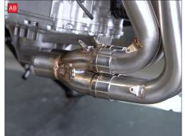
AC) Slide the secondary collector/ link pipe onto the primary collectors.
